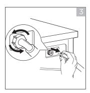
3. Unscrew the water supply hose from the backside of the machine. Pull out the filter with long nose pliers.
